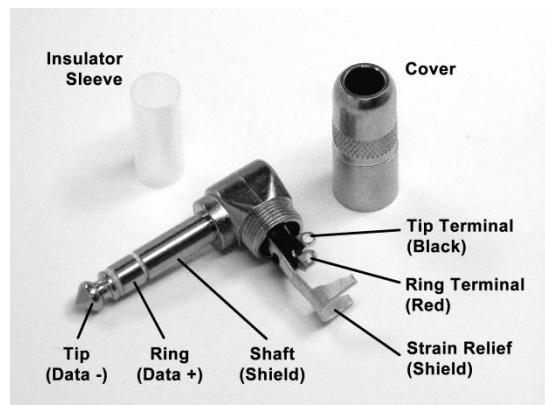
The other method requires the right-angle stereo plug assembly, which Electro-Mech provides with all hard-wired indoor scoreboard packages. In the case of shot clocks, there will be two plug assemblies to terminate the two cable runs required. The assembly consists of the main plug body, an insulating sleeve, and a cover.
