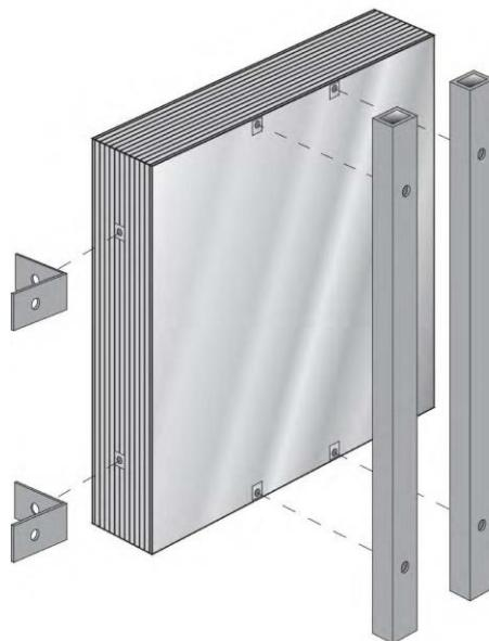
These mounting points are simple and generic enough to accommodate a variety of techniques for hanging the sign on assorted structures. The rear mounting points accept 1/2-inch 13 bolts and are provided to be used with vertical mounting structures running behind shot clock cabinet. In some cases, it may be easier to attach support pieces to the sides of the cabinets. Our side mounting points accept 3/8-inch 16 bolts.
