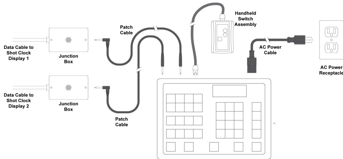
If your shot clock package includes Electro-Mech's ScoreLink RF Communications system, the power receptacle may be the only consideration on the control console side of the installation process. For details about ScoreLink, consult the documentation which ships with the product. Otherwise use the stereo patch cables to plug the controller into the junction boxes.
